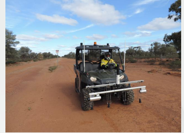
Performing gas leak detection services to ensure a pipeline is not leaking gas
